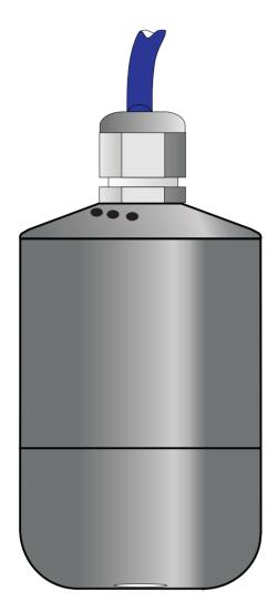
The Model 420 is a membrane covered galvanic oxygen probe with built-in two-wire 4-20 mA transmitter. The probe is connected to a DC supply and draws a current of between 4 and 20 mA corresponding to the oxygen concentration.
