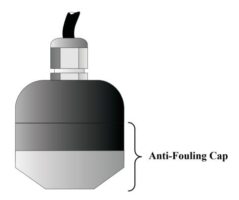
The **OxyGuard Anti-fouling Cap** is a cap that inhibits growths on the membrane of OxyGuard Standard Probes, especially probes used in sea water. The cap is essentially the same as the normal cap, but is fitted with a cone made from a specially developed alloy. The cone surrounds the membrane and is effective in inhibiting marine organisms from attaching to and growing on the membrane. Tests conducted in warm and cold sea water indicate that the cap is specially effective against barnacles.
