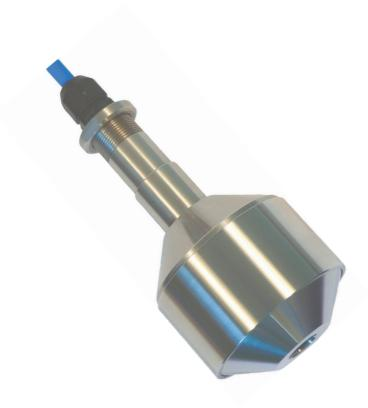
The OxyGuard probe is a membrane covered galvanic cell that generates an electrical signal proportional to the oxygen pressure it senses, no matter which medium it is placed in.
